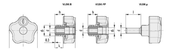
$\begin{array}{ll} D & = 63 \\ d1 & = 23 \\ d & 6H = M8 \\ h & = 18 \\ I & = \end{array}$
